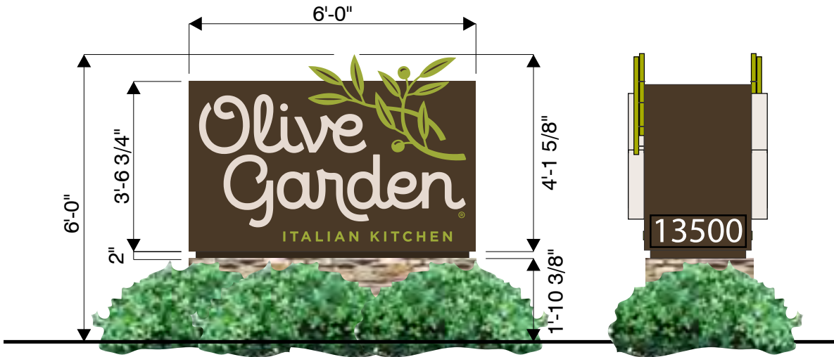
D 36 SF Monument ( Internally Illuminated Letters w/ LED ) Utilized Square Footage: 36 Scale: 3/8" = 1'
