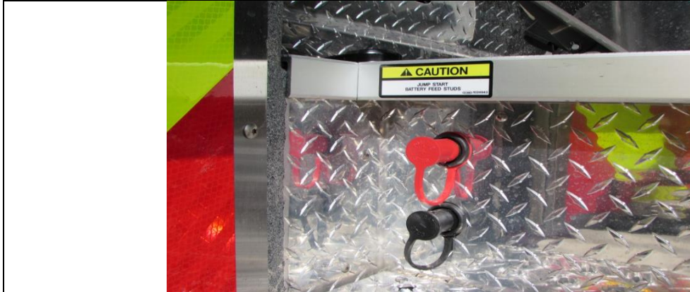
Jump Start Studs: Located below the drivers step inside the door.
