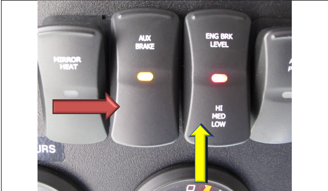
Jacobs(JAKE) Brake Controls Overhead Panel
