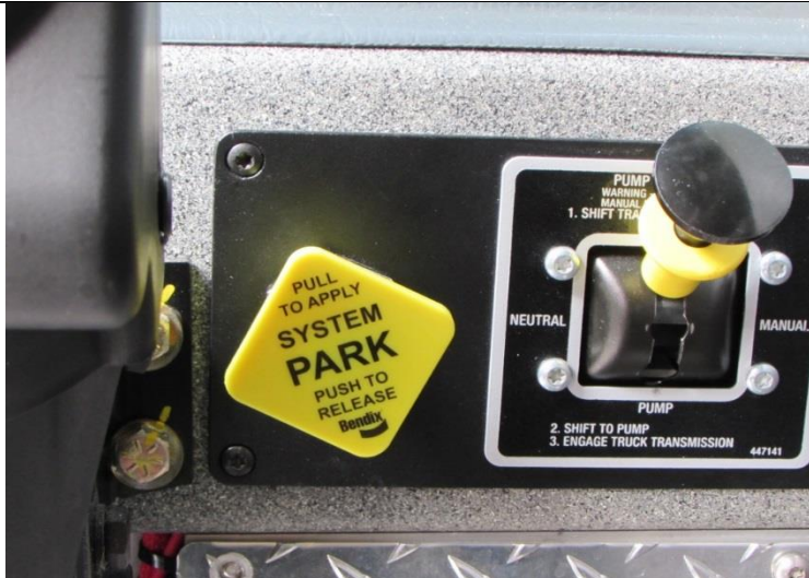
Parking Brake: Pull to apply and Push to release Please note the airbrakes will not release if the air pressure is below 70 PSI in the system
