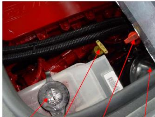
ENG COOLANT RESERVOIR, WASHER FLUID CAP AT FRONT OR RESERVOIR ENGINE OIL DIPSTICK TRANS FLUID DIPSTICK POWER STEERING RESERVOIR
