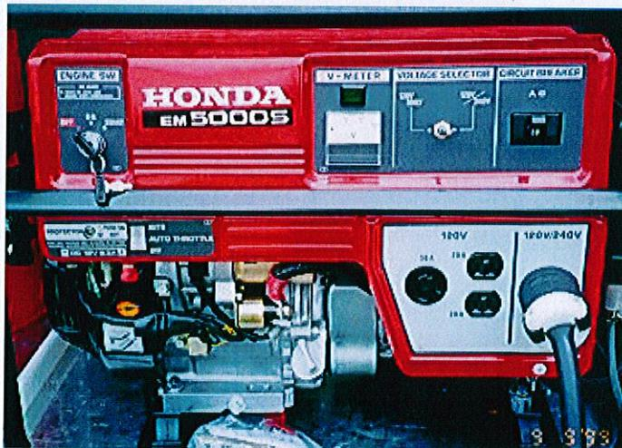
The generator draws its fuel supply from an integral 4.5 gallon fuel tank(gasoline) and has a 1.2 quart oil reservoir for 10W-30 or 10W-40 oil. The generator weighs 175 lbs. without fluids.
