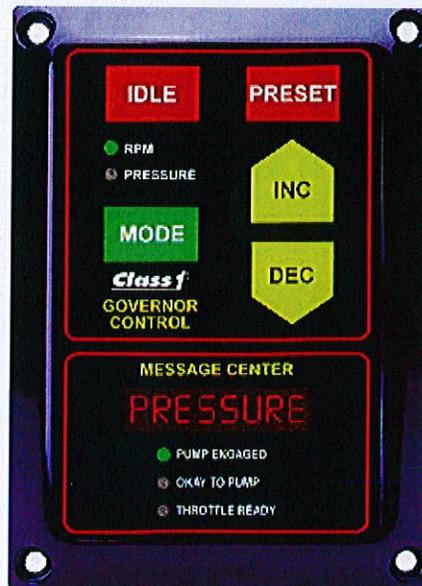
***RPM (throttle) mode*** - The RPM mode allows the operator to control engine speed like the old vernier throttles. This mode allows the operator to maintain a selected RPM. **The pressure governor (relief valve) feature does not function when the engine governor is in the RPM mode.** The anti-cavitation feature does not work in the RPM mode either. The driver operator can switch to
