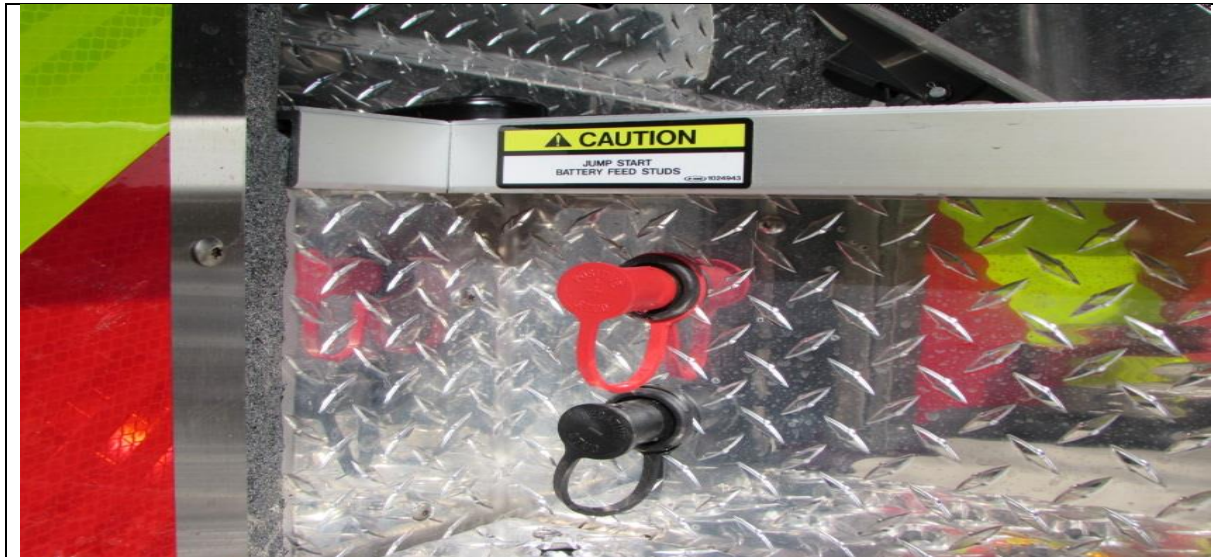
Jump Start Studs: Located below the drivers step inside the door.
