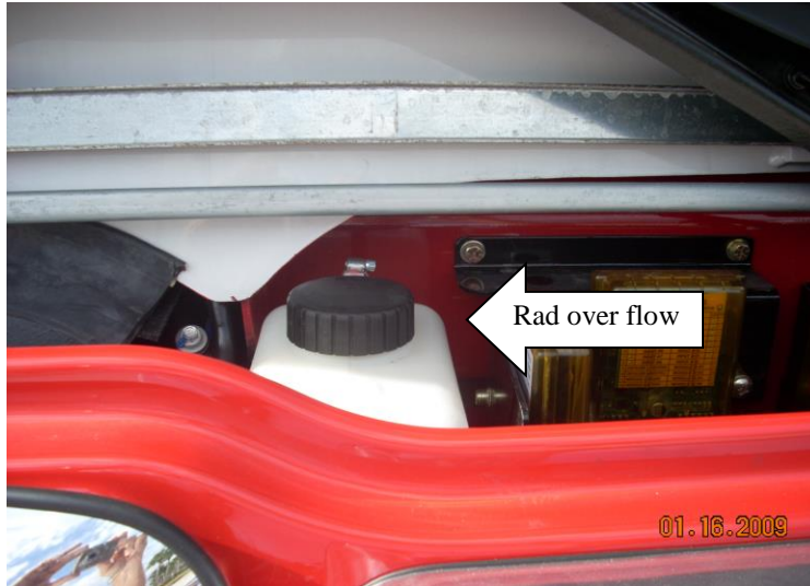
Radiator overflow reservoir is located under the hood left of center.
