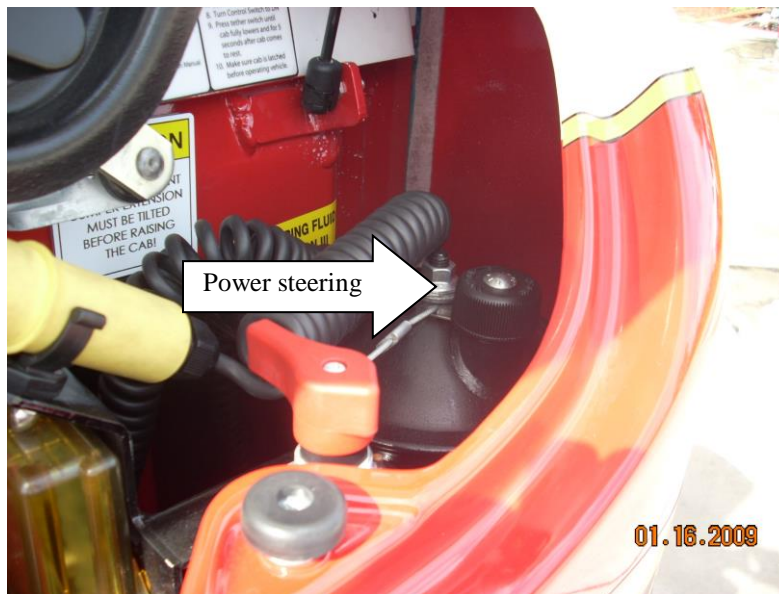
The power steering fluid reservoir is located on the driver's side under the hood.
