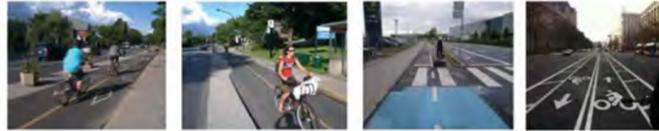
A cycle track is an exclusive bike facility that combines the user experience of a separated path with the on-street infrastructure of a conventional bike lane. A cycle track is physically separated from motor traffic and distinct from the sidewalk (NACTO).
