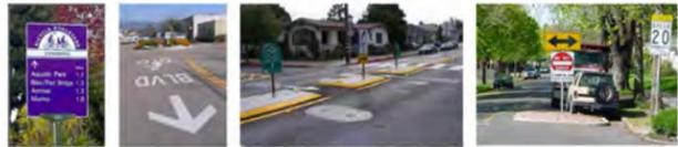
Bicycle boulevards are streets with low motorized traffic volumes and speeds, designated and designed to give bicycle travel priority. Bicycle Boulevards use signs, pavement markings, and speed and volume management measures to discourage through trips by motor vehicles and create safe, convenient bicycle crossings of busy arterial streets (NACTO).
