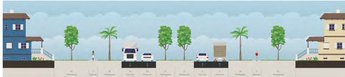
Sunset Strip - Existing Typical Cross Section
