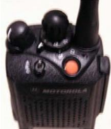
To activate the EAB, the operator simply depresses the EAB and holds it down for approximately 2 seconds until it rapidly beeps.
